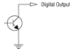
Figure 64: Open Collector Digital Output.
