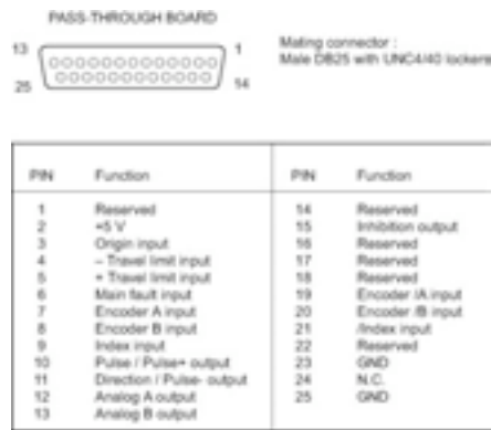
Figure 75: DRV00 Pass-Through Connector.
