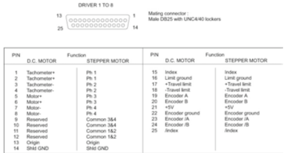
Figure 71:XPS-DRV01 Motor Driver Connectors.
