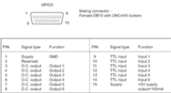
Figure 68: GPIO3 Digital I/O Connector.
