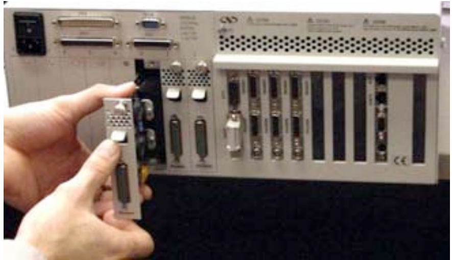
Figure 11: Installing Driver cards.
