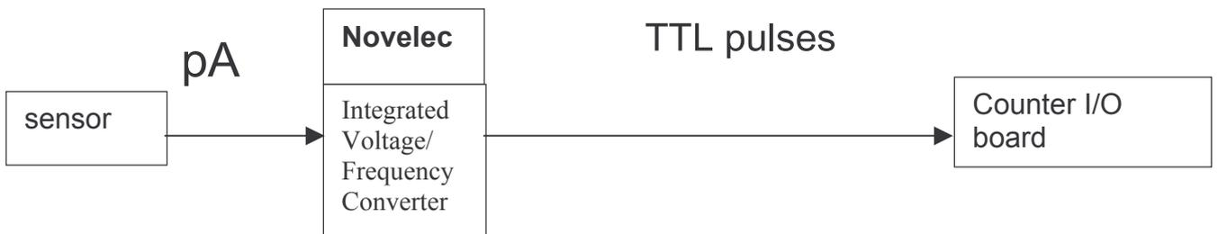
On a few SOLEIL beamlines, Novelec electrometers are used for pico current acquisitions. The main difference is that all models integrate a voltage/frequency converter.
